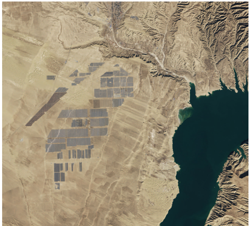
February 2017, Longyangxia Dam Solar Park in China, 850 MW of capacity. Image acquired by the Operational Land Imager (OLI) on Landsat 8. By January 5, 2017, solar panels covered 27 square kilometers (10 square miles) of Qinghai province. According to news reports, there were nearly 4 million solar panels at the site in 2017.
